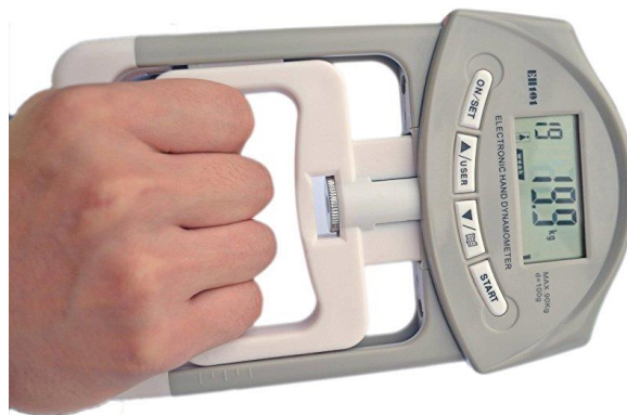
Figure 2: Digital Jamar Handgrip Dynamometer
